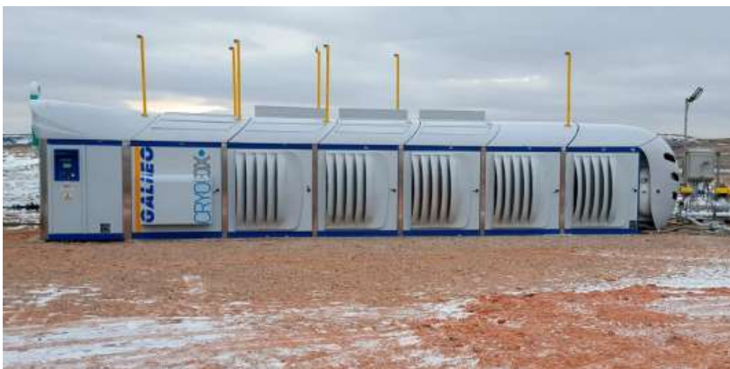
Figure 11. Cryobox® LNG production station [Galileo Technologies 2017].
